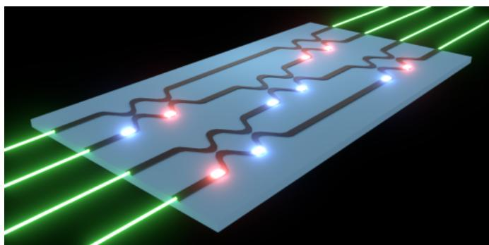
**Figure description** - Researchers have shown a neural network can be trained using an optical circuit (blue rectangle in the illustration). In the full network there would be several of these linked together. The laser inputs (green) encode
