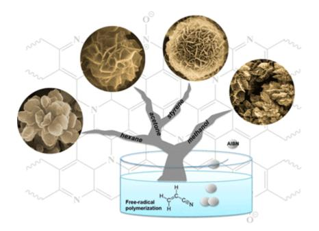
**Synthesis of carbon flower superstructures:** This schematic image shows the variety of structures formed by varying the solvents for this simple polymerization process. Additional shapes and pores can be introduced by incorporating other co-monomers.
