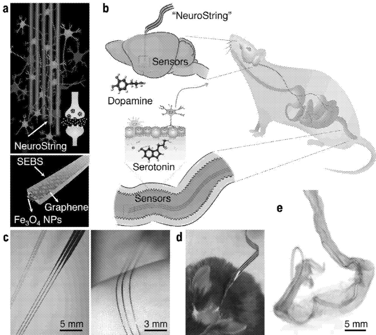
**Figure 1** Laser printed "**NeuroString**" for brain and gut neurotransmitter sensing. A) Schematic of a soft brain implant for neurotransmitter sensing. B) Illustration of NeuroString implanted in brain and colon. C) 3 channel NeuroString. D) NeuroString implanted in mouse. E) X-ray computed tomography of NeuroString in mouse colon.
