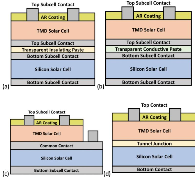
**Figure description** - Schematics of (a) mechanically stacked, four-terminal, (b) mechanically stacked, three-terminal, (c) monolithically integrated, three-terminal, and (d) monolithically integrated, two-terminal TMD/Si tandem solar cells
