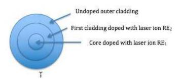
**Cross section of ASF cooled optical fiber** – The fiber to be cooled is doped with laser ion RE<sub>1</sub>. Anti-Stokes fluorescence cooling goes on in the cladding doped with laser ion RE<sub>2</sub>. Due to refractive index differences the core and first cladding are optical waveguides. In order to maintain uniform cooling, doping concentration and cladding diameter can vary along the length of the cladding. The fiber can also be
