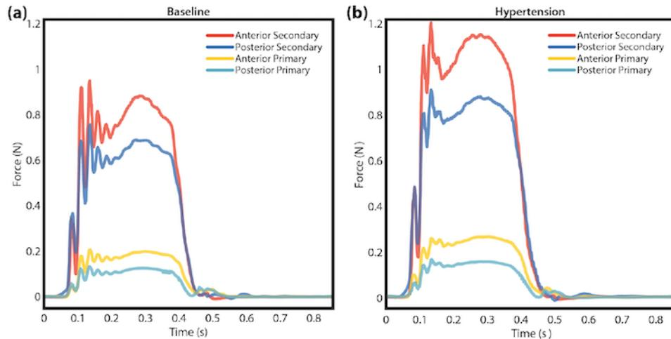
Force tracing of chordae tendineae at baseline (left) and during hypertensive conditions (right), demonstrating proper function of FBG sensor.
