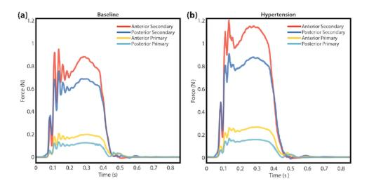
Force tracing of chordae tendineae at baseline (left) and during hypertensive conditions (right), demonstrating proper function of FBG sensor.
