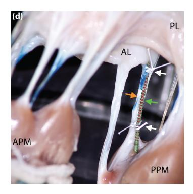
Prototype FBG-based force sensing nechord (green arrow) implanted ex vivo via suture (white arrow) to measure the chordae of interest (orange arrow). APM: anteriolateral papillary muscle; PPM: posteriomedial papillary muscle, AL: anterior leaflet.
