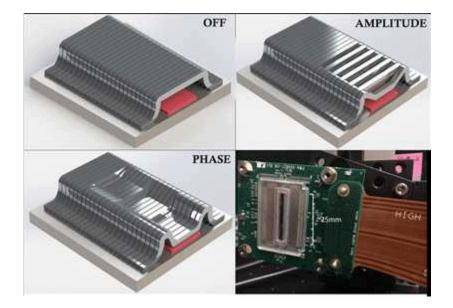
**Phased Array for Random Access Scanning:** Model of phased array with silicon ribbons in passive state (off) and active operation (amplitude and phase). By controlling the ribbon with small voltages, the device acts as a diffraction grating for pulsed laser light.
