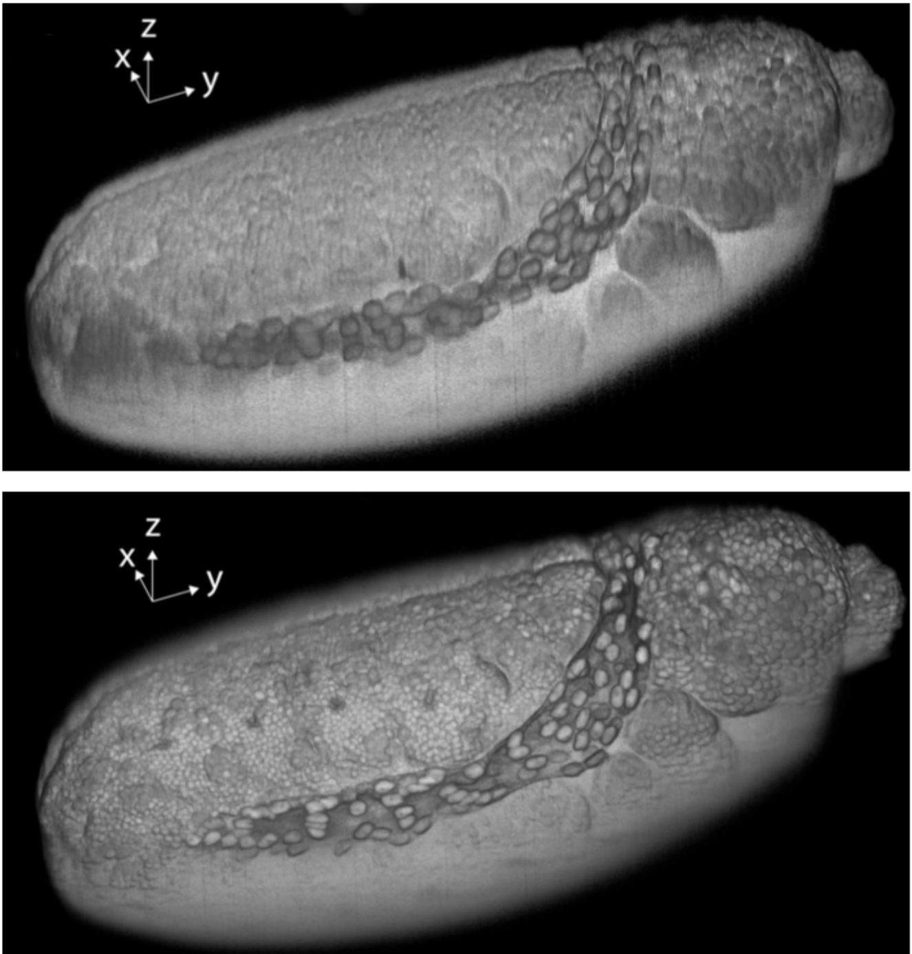
Fig. 2 Drosophila embryo 3D images showing the surface of the reconstructed 3D volumes with rolling shutter widths of 1625 (top) and 65 \mu\text{m} (bottom), respectively.
