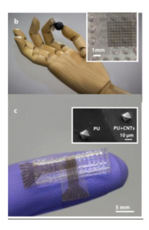
**Figure description -** b) Optical image of a fabricated e-skin and close-up view on the hills and electrodes (inset). c) Optical image showing the CNTs-PU (polyurethane) interconnects for signal recording with LCR (inductance-capacitance-resistance) meter and SEM picture of the top e-skin layer with molded pyramids, showing CNTs-PU and PU areas (inset).
