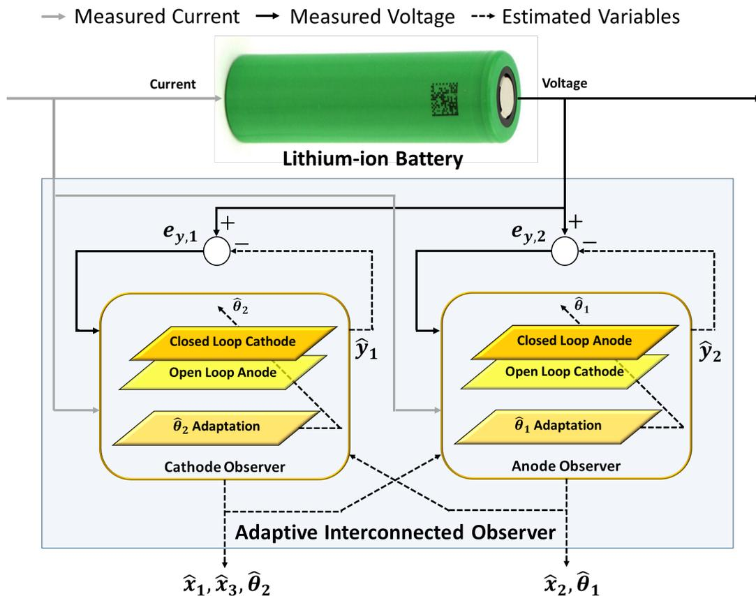
**Figure description** - The adaptive interconnected observer structure consists of a cathode observer and an anode observer that update each other via a bidirectional interconnection for the combined estimation of lithium concentration in cathode ( $\hat{x}_1$ ) and anode ( $\hat{x}_2$ ), the total cell capacity ( $\hat{x}_3$ ), and aging-sensitive parameters like the anode diffusion coefficient ( $\hat{\theta}_1$ ) and the SEI layer ionic conductivity ( $\hat{\theta}_2$ ).
