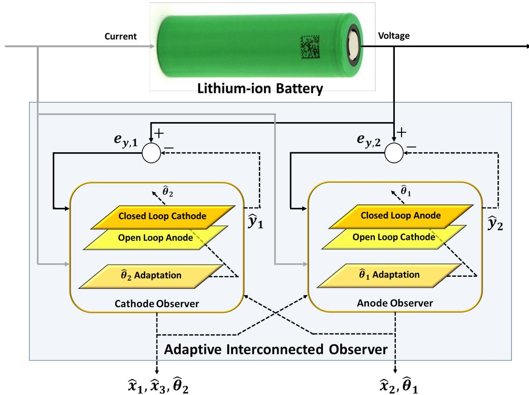
**Figure description** - The adaptive interconnected observer structure consists of a cathode observer and an anode observer that update each other via a bidirectional interconnection for the combined estimation of lithium concentration in cathode ( $\hat{x}_1$ ), anode ( $\hat{x}_2$ ), the total cell capacity ( $\hat{x}_3$ ), and aging-sensitive parameters like the anode diffusion coefficient ( $\hat{\theta}_1$ ) and the SEI layer ionic conductivity ( $\hat{\theta}_2$ ).
