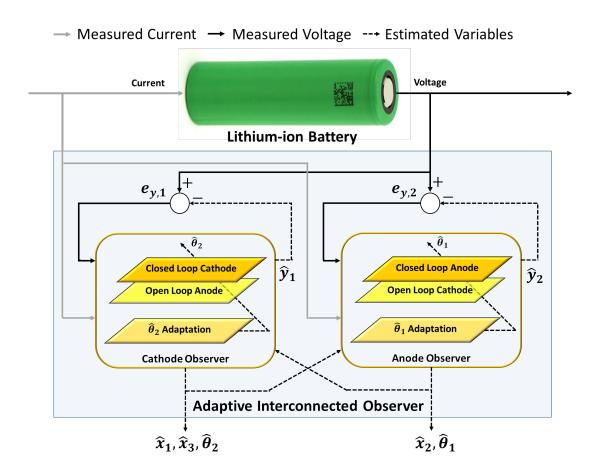
**Figure description -** The adaptive interconnected observer structure consists of a cathode observer and an anode observer that update each other via a bidirectional interconnection for the combined estimation of lithium concentration in cathode  $(x_1^2)$  and anode  $(x_2^2)$ , the total cell capacity  $(x_3^2)$ , and aging-sensitive parameters like the anode diffusion coefficient  $(?_1)$  and the SEI layer ionic conductivity  $(?_2)$ .
