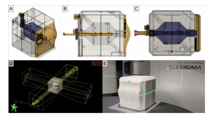
Design and development of a QA phantom to quantify the spatial accuracy of a linear accelerator- based single-isocenter, multitarget cranial radiosurgery system ( **A-C**). (**D**) Eclipse treatment plan portal fields. (**E**) 3D printed QA phantom on Varian Truebeam (Varian Medical Systems, Palo Alto, CA).
