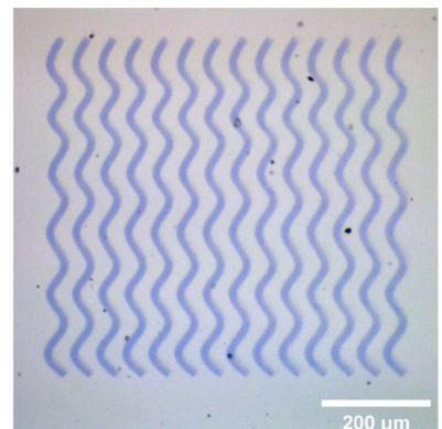
**Figure 1 Photo patterned PEDOT** showing possible minimal feature sizes with about 2  $\mu\text{m}$  minimum size.
