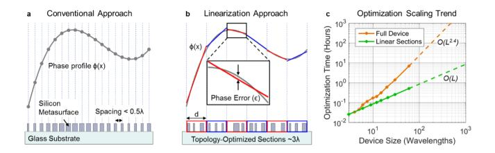
**Figure 1**. Metasurface design approaches. a) Conventional approaches sample the desired phase profile at discrete points and specify phase shifting elements to form a nanoscale phased array. b) **Fan Lab approach** is to divide the desired phase profile into wavelength-scale, linear sections and use topology optimization to
