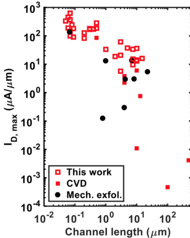
Figure 3 Flexible MoS<sub>2</sub> Devices Benchmarking
