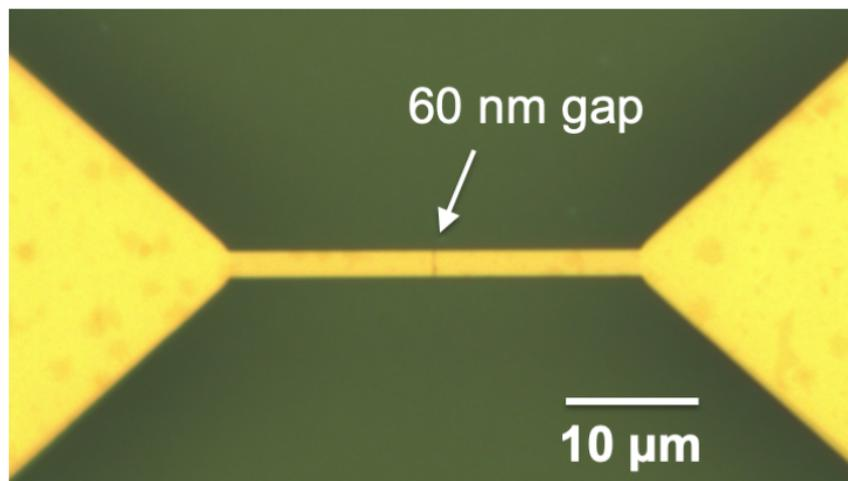
Figure 2 Short Channel Top-Gated Staggered MoS<sub>2</sub> FETs
