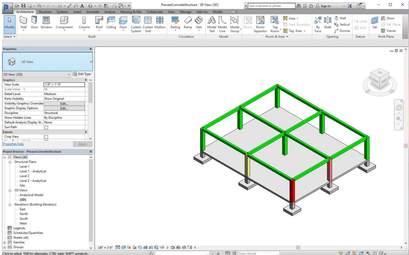
**Future deterioration display risk map of parking structure.** In this example, colors indicate increasing deterioration risk - i.e., the probability that each element will exhibit corrosion-induced surface cracking 25?years in the future (red shading indicates highest probability, pink shading indicates medium probability, yellow shading indicates minor probability, and green shading indicates low probability of surface cracking). Image courtesy of Blume Lab.
