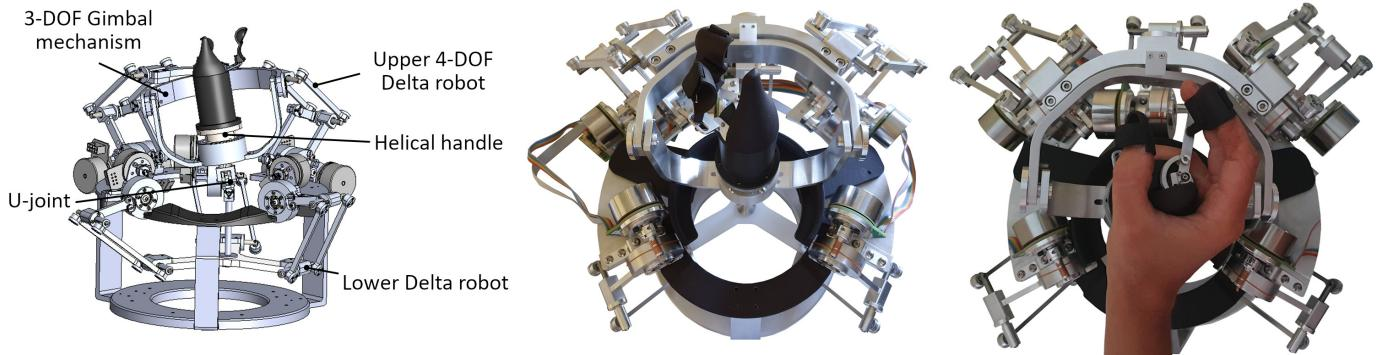
**Compact and High-Fidelity Device for Versatile Haptic Teleoperation** The mechanical transparency of the design and its novel paired parallel structure meet the challenge of accuracy, stiffness, and haptic capability required in remote tasks.
