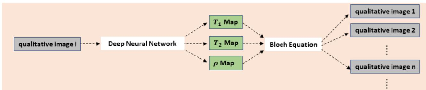
**Figure description** - Scheme of retrospective tuning of tissue contrast in MRI: from a single image, tissue relaxation parametric maps are derived and used to calculate images presumably acquired using other imaging protocols, providing a wide spectrum of tissue contrasts.
