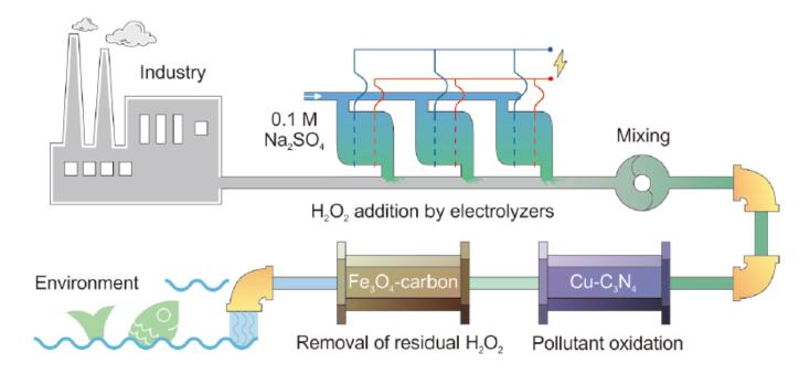
Photo description: Schematic of the wastewater treatment system, specifically addressing production and activation of H2O2.
