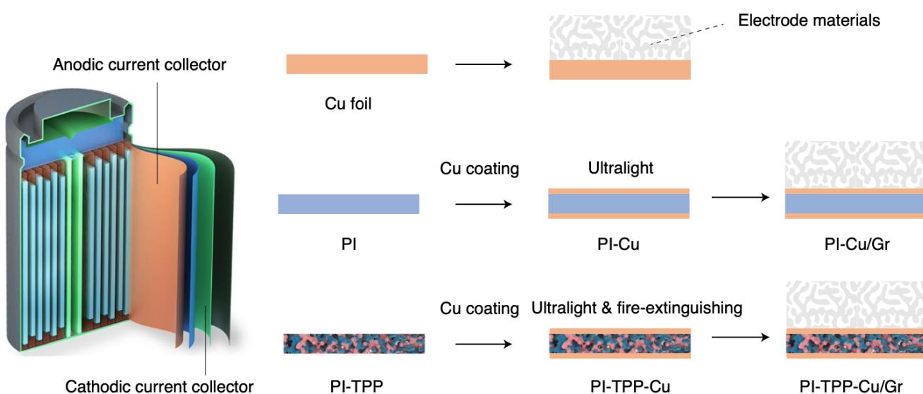
**Figure 1** Current collector designs. Top) Heavy and bulky pure Cu current collectors. Middle) Lighter Polyimide-Copper current collector. Bottom) **Stanford's Yi Cui Lab developed PI-TPP-Cu Current Collector**. Ultralight, flame retardant current collector design with ultrathin metal layers on both sides of a triphenyl phosphate (TPP) flame retardant embedded polyimide layer. Schematic courtesy the Yi Cui Lab.
