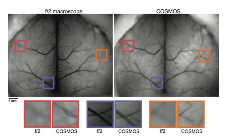
Merged image quality vs. a conventional macroscope with the same light throughput. COSMOS yields high quality extended depth of field. (image credit: the inventors)
