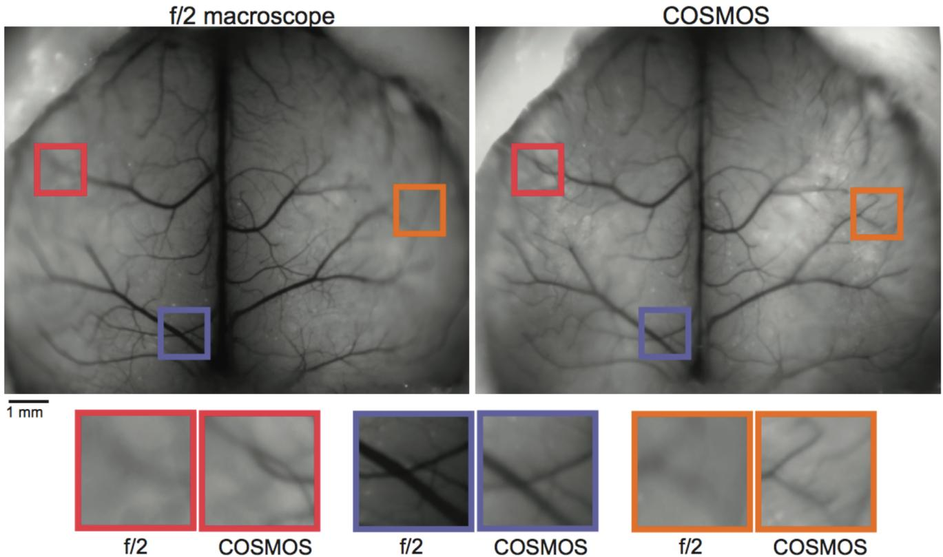
Merged image quality vs. a conventional macroscope with the same light throughput. COSMOS yields high quality extended depth of field. (image credit: the inventors)
