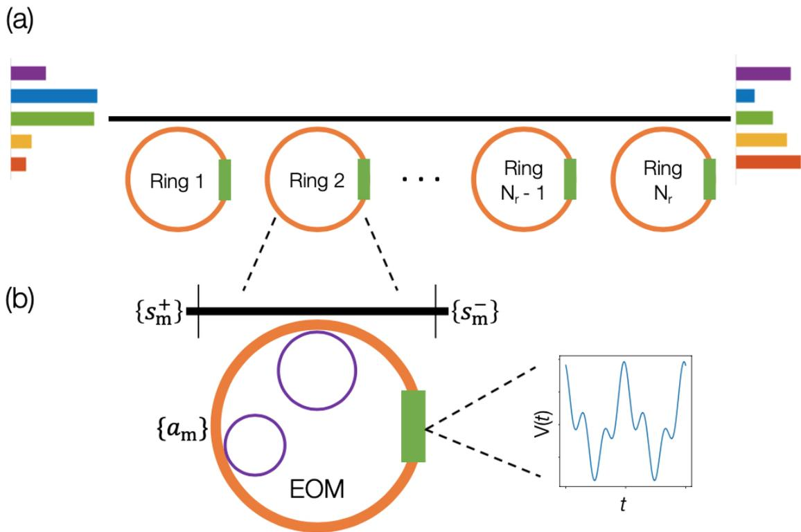
**Schematic of the Frequency Changing & Tuning Photonic Device**
