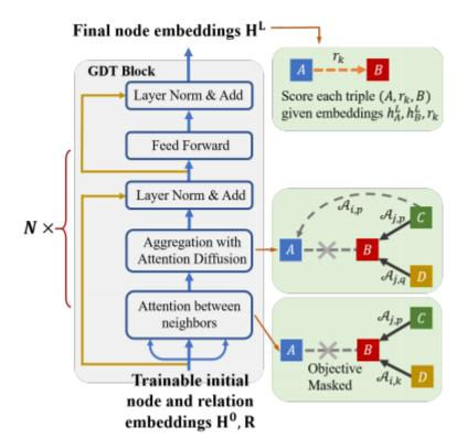
**GDT architecture**. Each GDT block consists of attention computation, attention diffusion, layer normalization, feed forward layers, and 2 residual connections for each block. GDT blocks can be stacked to constitute a deep model. As illustrated on the right, context-dependent attention is achieved via the attention diffusion process. Here A, B, C, D? V are nodes in the graph. (image credit: the inventors)
