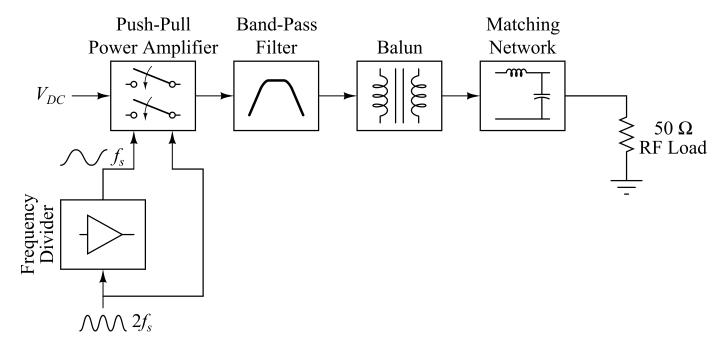
Photo description: Block diagram of the wideband resonant inverter.
