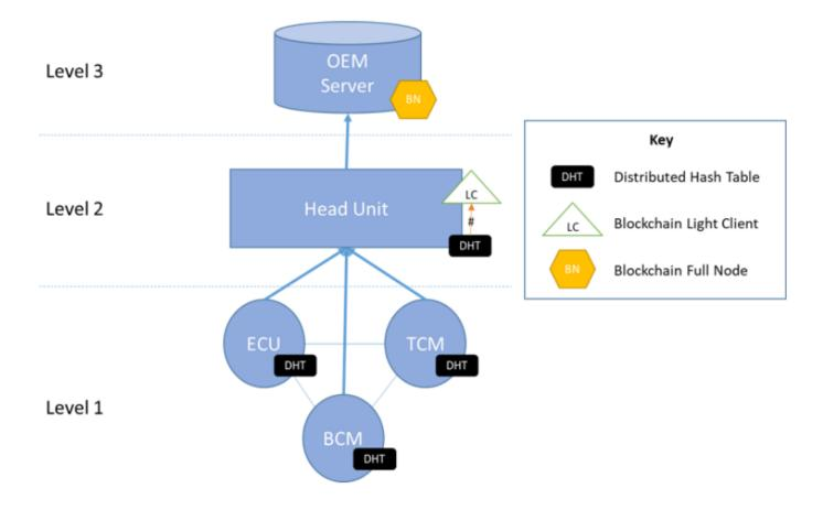
This three-layered architecture blends a DHT implementation with a blockchain implementation, to gain the benefits of both technologies without imposing undue computational burden on constrained compute modules (image credit: the inventors)
