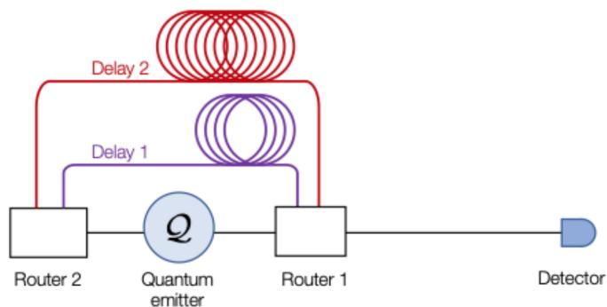
**Figure description** - A schematic illustration of the apparatus required to implement our protocol. Propagating modes, e.g., photons or phonons, interact with the emitter three times, followed by an adaptive measurement.
