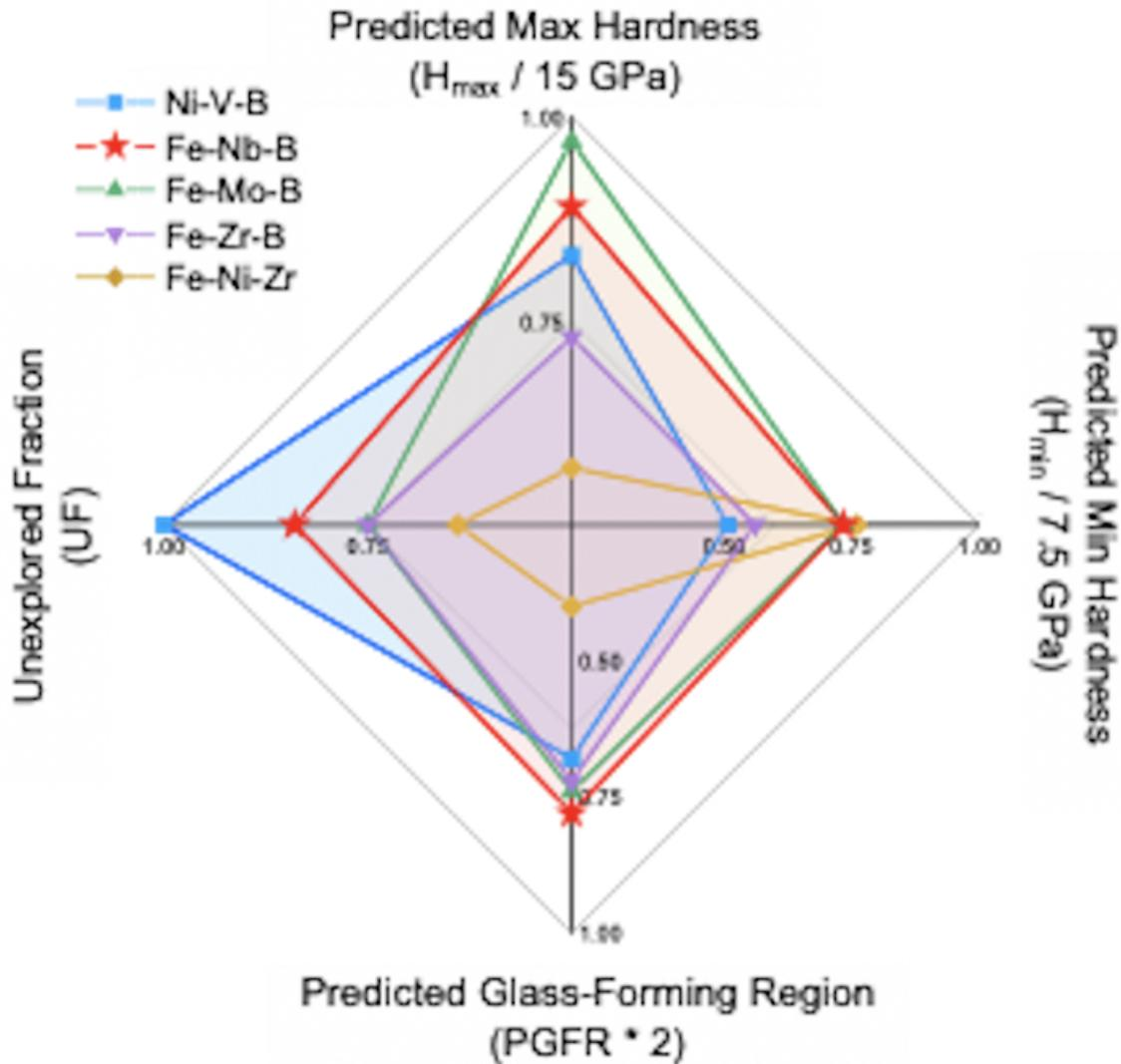
**Figure description** - Top 5 candidate MPEA ternary systems for exploration. Each axis represents 4 desired characteristics of 5 ternary systems (individual axis are normalized 1 to reduce complexity of the plot).
