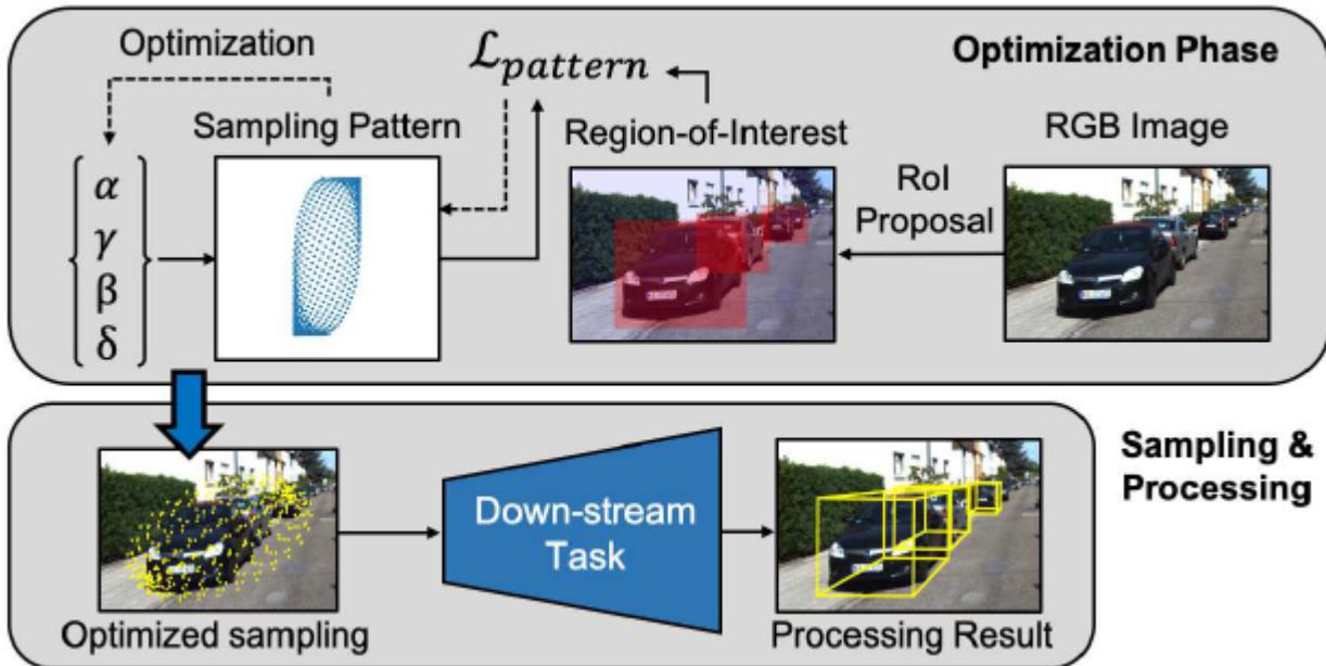
Photo description: Schematic pipeline of the optimization framework using 3D object detection as an example target task. Credit: Sun et al. arXiv (2021).
