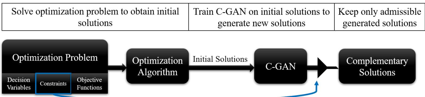
Photo description: Overview of the proposed algorithm for using a C-GAN to complement an optimization algorithm on a high-dimensional nonlinear optimization. Credit: Kalehbasti et al. arXiv (2021)
