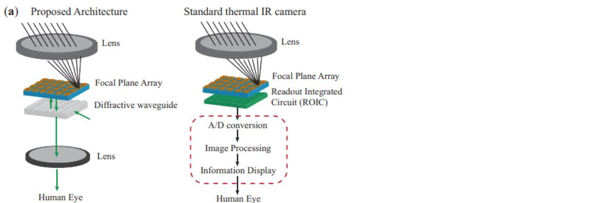
The proposed architecture is schematically shown in comparison to the standard thermal IR imaging system. Seen in the red dotted lines are system parts eliminated
