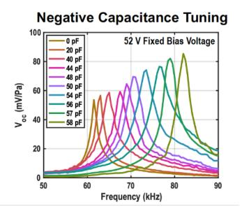
Figure Description: Via the negative capacitance tuning technology described, the inventors are able to attain high sensitivity at all frequencies (source: inventors).
