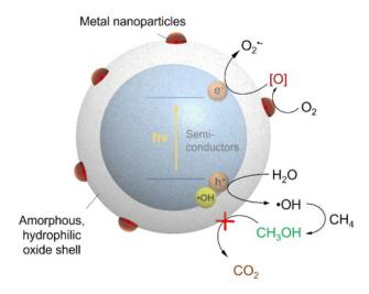
Structure of the new photocatalysts for methane partial oxidation at room temperature. The researchers have shown that enclosing photocatalysts with transport selective structures is a generalizable strategy to achieve high selectivity and activity simultaneously in photochemical alkane oxidation reactions. (image credit: the inventors)
