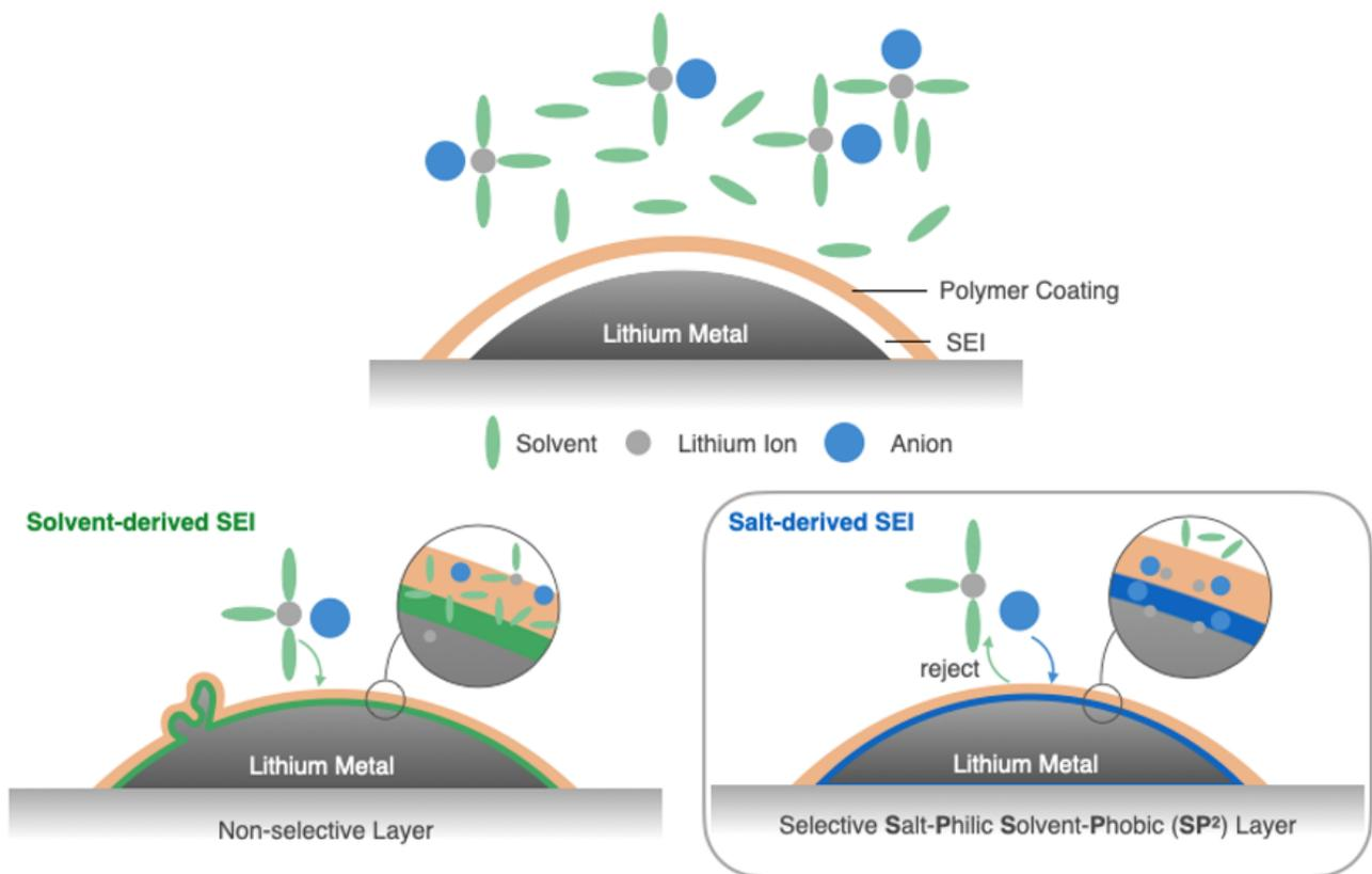
**Figure 1** A Salt-Philic Solvent-Phobic (SP<sup>2</sup>) polymer coating on Li metal anode induces salt derived solid electrolyte interface formation. (Image courtesy the Zhenan Bao Group and the Yi Cui Group)
