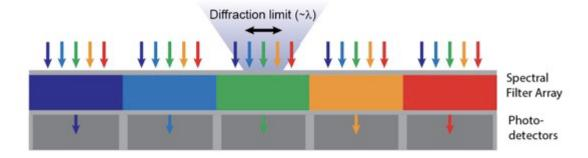
(b) Spectral router: Highly efficient routing of spectral components in (sub)wavelength footprint
