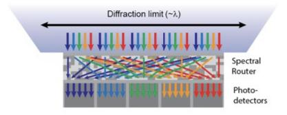
(c) Example spectral router with 6 spectral channels in the visible wavelength range
