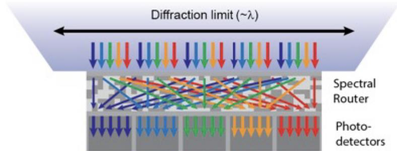
(c) **Example** spectral router with **6 spectral channels** in the **visible wavelength range**
