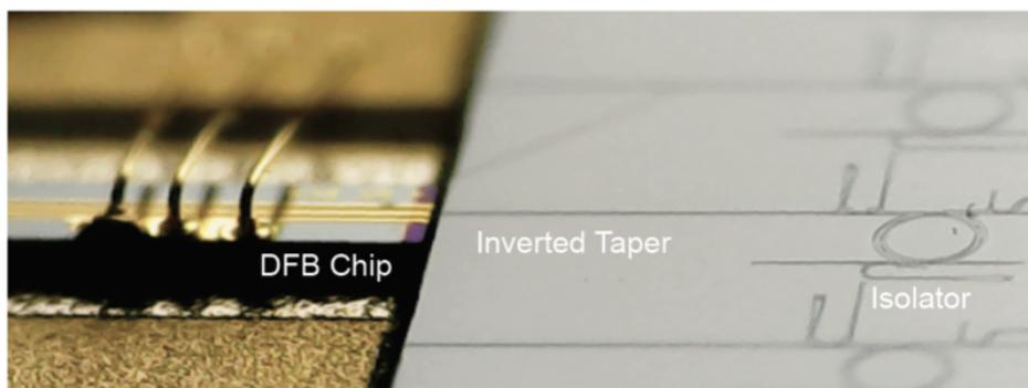
Figure 1 Optical image of hybrid integration of DFB laser with the isolator
