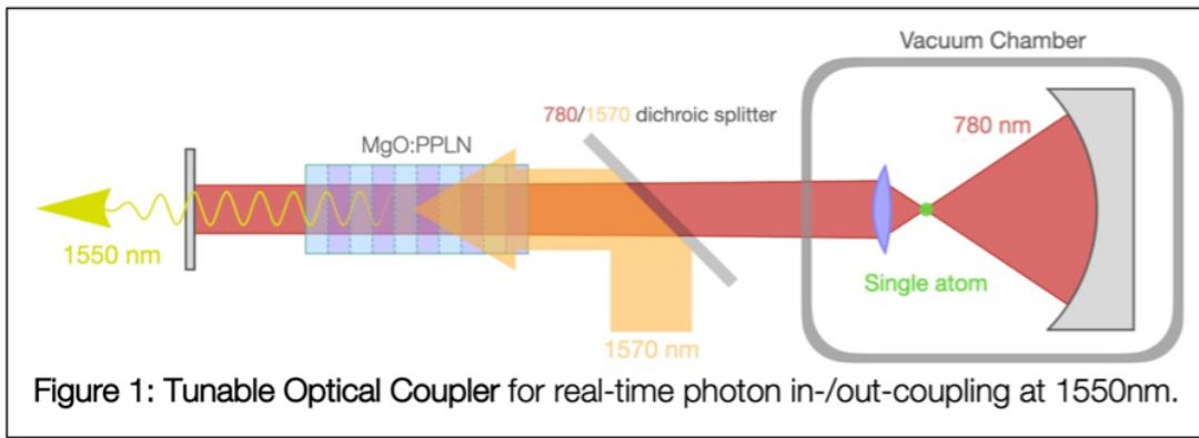
Figure 1: Tunable Optical Coupler for real-time photon in-/out-coupling at 1550nm.
