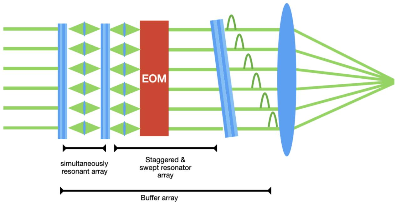
**Figure 1 Buffer array with coupled cavity arrays + EOM**
