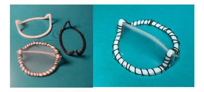
Figure description: Prototypes of bi-leaflet stent for modular bioprosthetic valve using biocompatible polyurethane RPU70 resin in Carbon 3D printer. (Image credit: https://doi.org/10.1016/j.xjon.2023.04.007)
