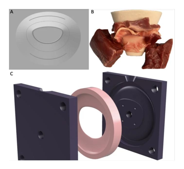
Figure description: **A)** A computer-aided design rendering of the 3D-printed mitral annular dilator. **B)** The annular dilation device placed across a juvenile porcine mitral valve to induce annular dilation. **C)** Exploded view of the elastic dilated mitral mount produced using 3D-printed molds. (Image credit: https://doi.org/10.1186/s12872-022-02515-x)
