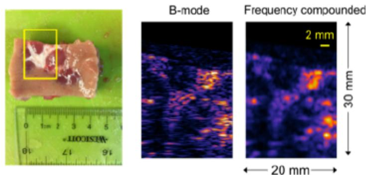
**Figure description** - Use of Fourier-filter speckle reduction method to image a piece of porcine kidney. Figure shows optical image (left panel) of a portion of kidney tissue imaged by ultrasound. The minor and major calyces appear white in the optical image. The same features can be identified in the conventional B-mode image (middle panel). The frequency compounded image shows reduced speckle while maintaining good spatial resolution.
