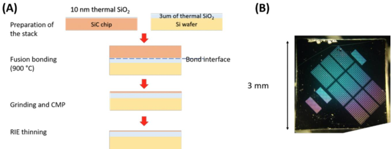
Figure 1: (A) Illustration of the process flow. (B) Image of a chip with 4H-SiCOI photonic devices. Note: for industry scaling, Si handle wafers (as opposed to SiC) would be used, because thermal stresses during and after bonding could detach the SiC wafer bonded to SiO<sub>2</sub> on Si.
