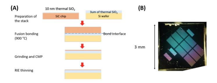
Figure 1: (A) Illustration of the process flow. (B) Image of a chip with 4H-SiCOI photonic devices. Note: for industry scaling, Si handle wafers (as opposed to SiC) would be used, because thermal stresses during and after bonding could detach the SiC wafer bonded to SiO2 on Si.
