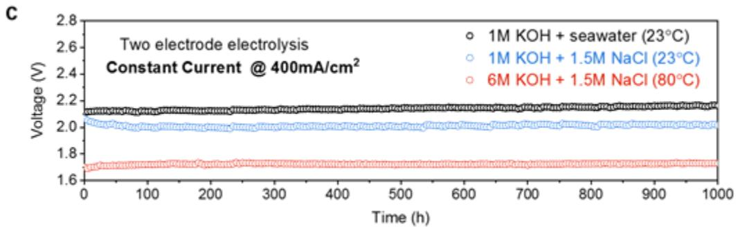
**Sustained, energy efficient seawater splitting continuously over 1000 hours.** Durability test for electrolysis in an alkaline seawater electrolyte (black), an alkaline simulated seawater electrolyte with near saturated salt concentration (blue) and industrial electrolysis conditions (red).
