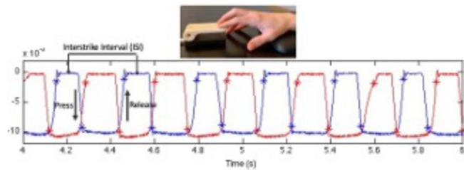
**Figure 1** - Upper panel: photo of a digitography device with the index and middle fingers placed on the levers. Lower panel: example of alternating full amplitude presses and releases by the adjacent fingers over time. Each finger is denoted by red or blue trace respectively. The press and release phases are labelled with arrows. The y-axis is amplitude; the x-axis is time. The interstrike interval (ISI) is the time it takes to complete a full cycle of the task with one finger.
