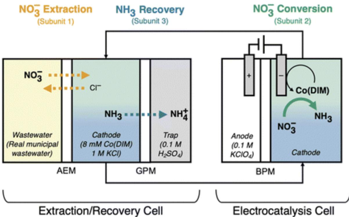
**Electrocatalyst-in-a-box (ECaB) Schematic**
