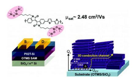
A conjugated polymer made with the novel siloxane-terminated solubilizing group exhibited a pi-pi stacking distance of 3.58 Angstroms which led to superior performance in a thin film field effect transistor (maximum mobility of 2.48 cm2/Vs).
