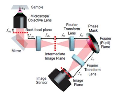
Phase Mask can be simply implemented with a tilted light-sheet microscope (LSM)
