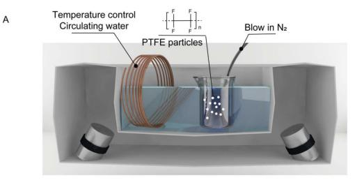
**Figure description:** Schematic representation of the experimental setup, synthesizing ammonia ( $\mathrm{NH}_3$ ) by bubbling nitrogen ( $\mathrm{N}_2$ ) gas into bulk liquid water containing polytetrafluoroethylene (PTFE) particles suspended with the help of a surfactant at room temperature.
